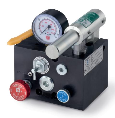
Output port:1/2" BSPPressure switch port (2 times):1/4" BSPSuction port:1/4" BSPPressure range:0-100 bar (0-1450 psi)Return port:1/4" BSPOil Viscosity:(25-60) cSt. bei 40°C (15-35 cSt. at 120°F)
